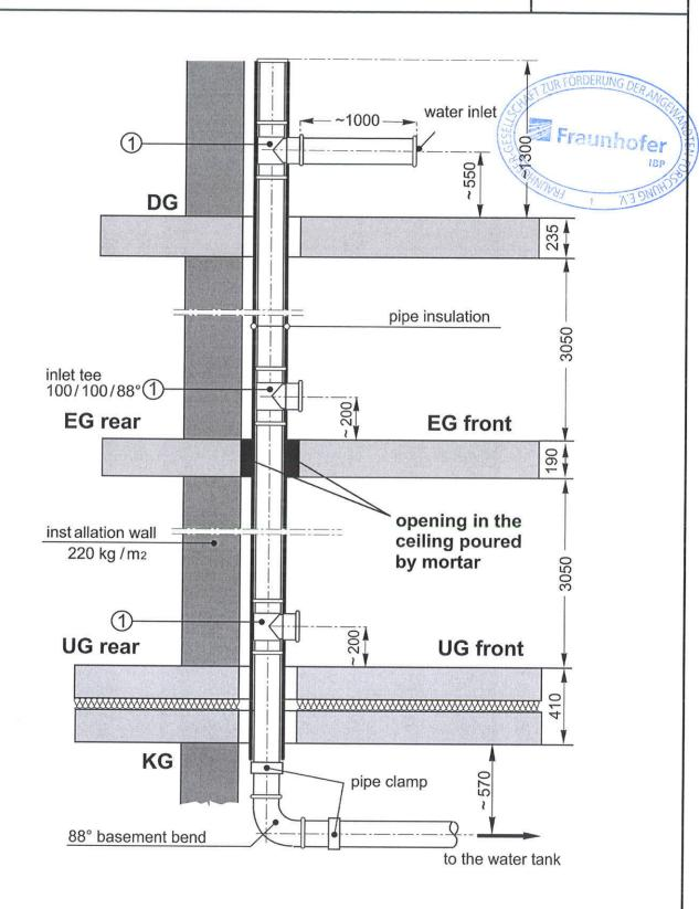
Installation plan of the waste water system (plastic pipes, HT, without pipe clamps) with the Insulating tube for wastewater installation systems "ENERGOFLEX ACOUSTIC", manufacturer: Rols Isomarket (drawing not to scale, dimensions in mm).
